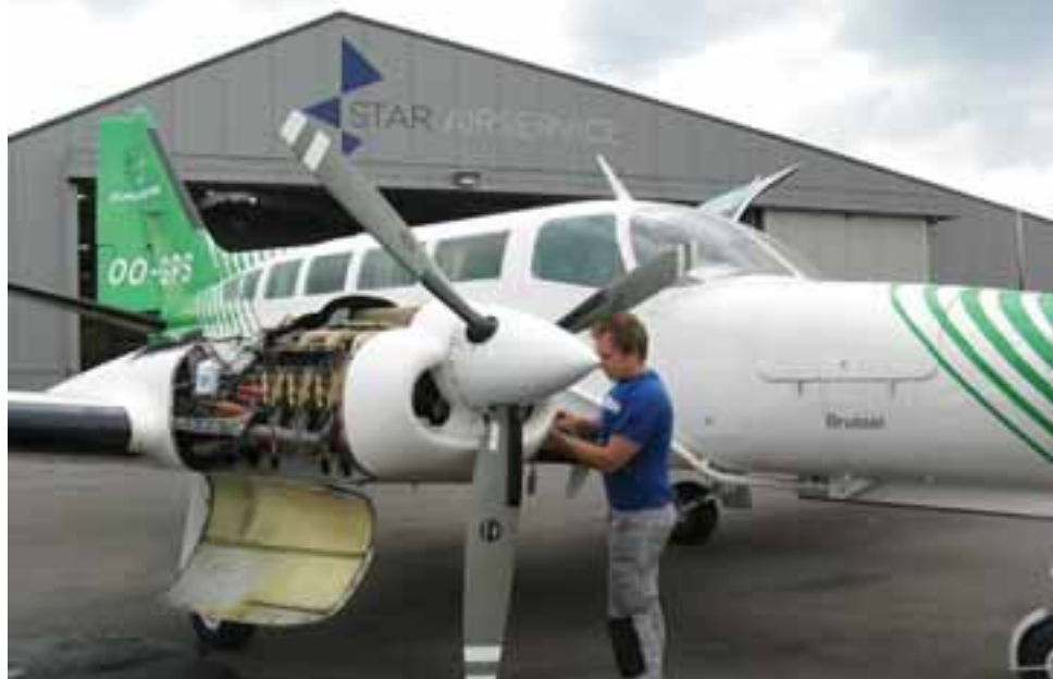
A Star Airservice technician prepares this Cessna 404 for an engine run.
