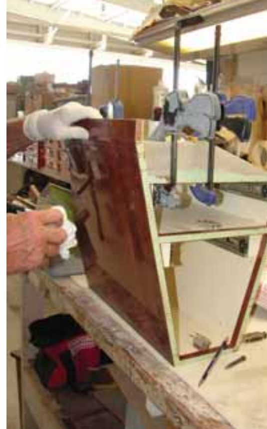
Wood veneers are very thin and often times damage results in replacement of the veneer.
