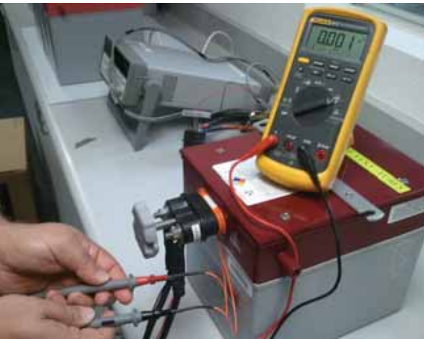
The parasitic drain of an aircraft battery can be directly measured with a digital multimeter (DMM) equipped with an ammeter function. Photos courtesy of Concorde Battery Corporation.
