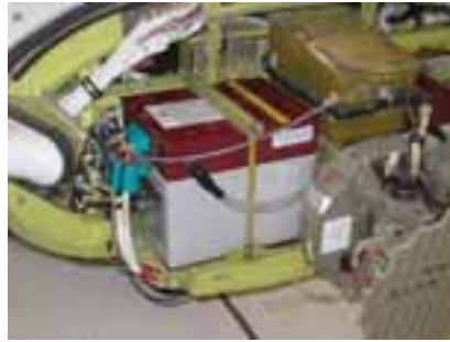
Concorde RG-390E battery installed in Sikorsky S-76B helicopter.
