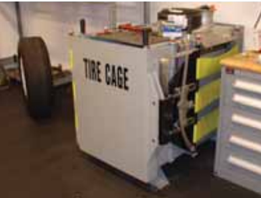
A tire cage is highly recommended for safely inflating aircraft tires. Photos provided by Peter Zeeb, Caesars Entertainment Inc.
