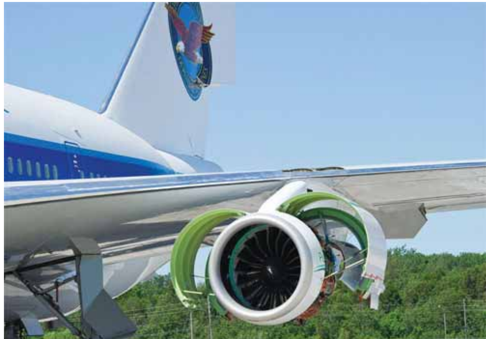
PW1500G mounted on the P&W B747SP flying test bed.
