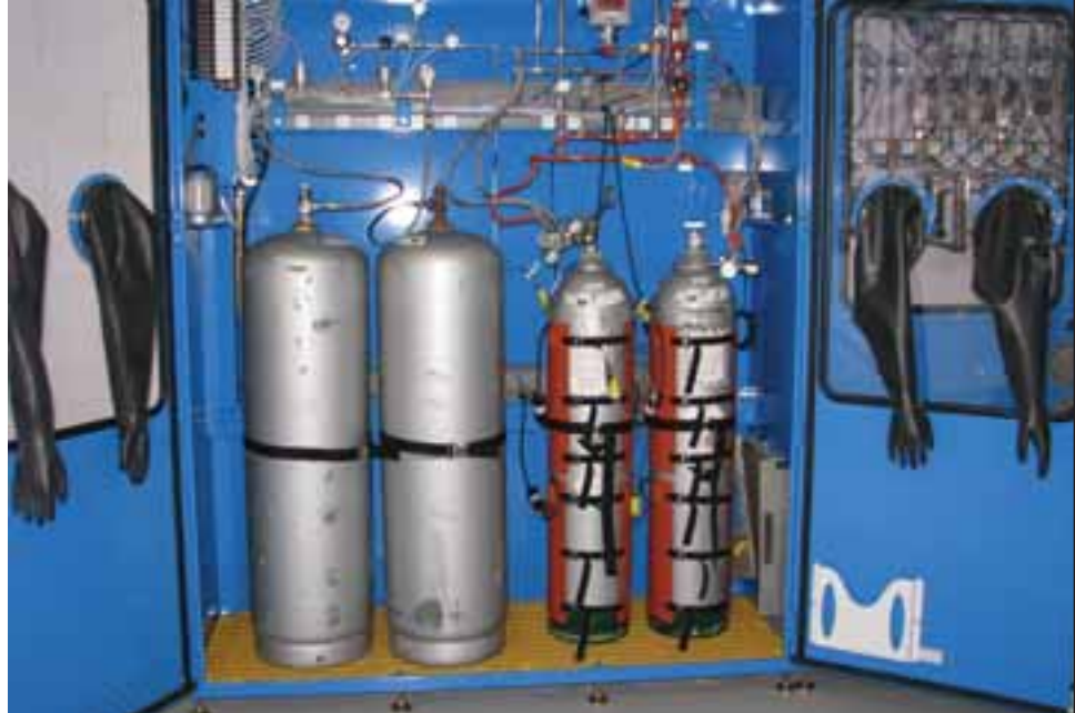
During processing, HF and H2 gas are introduced into the system through precision metering so time and gas concentrations can be precisely controlled.
