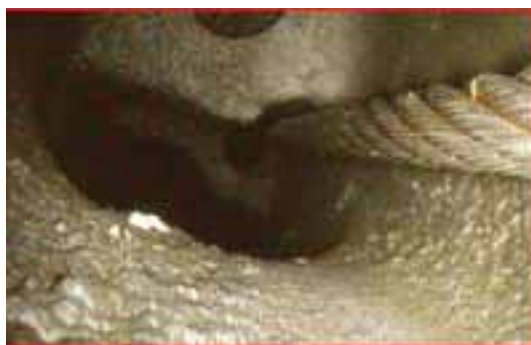
Miss-routed cable inside in the center of the column assembly. Control movement caused it to cut into the magnesium casting.
