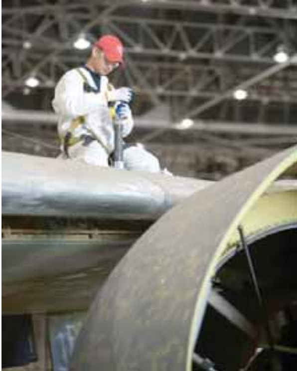
NAAS specialist preparing to seal a KC135 wing fuel tank.
