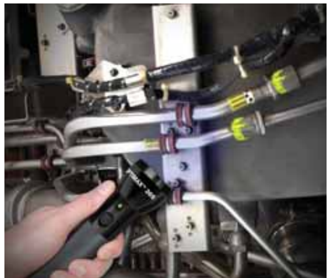
Aero-Brite universal fluorescent leak detection dye used to locate fuel leaks shows a yellow color for easy identification of leaks.
