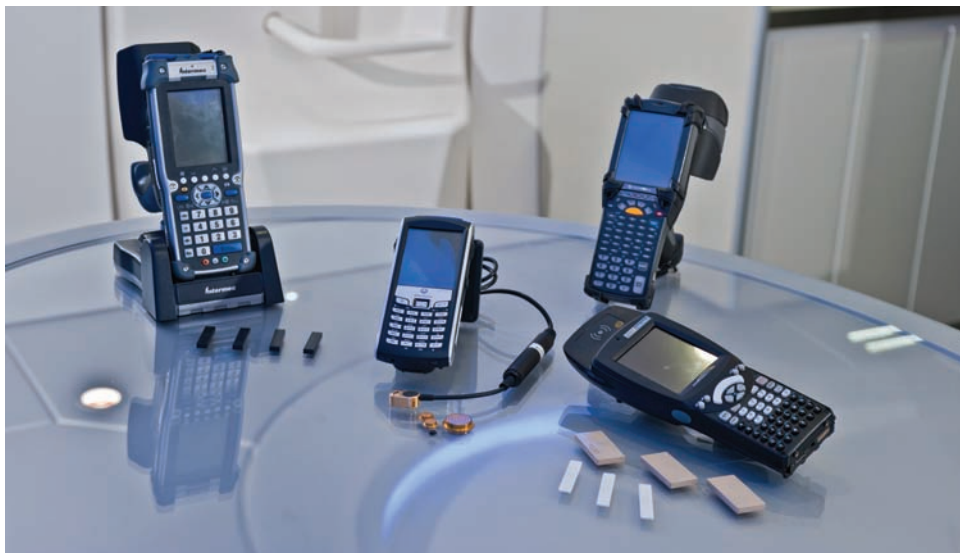
RFID tags and the associated reader/writers are available in a variety of shapes and sizes. Photo courtesy of The Boeing Company.
