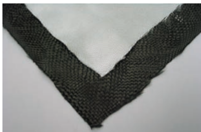
Black colored carbon fiber cloth and lighter colored fiberglass cloth.
