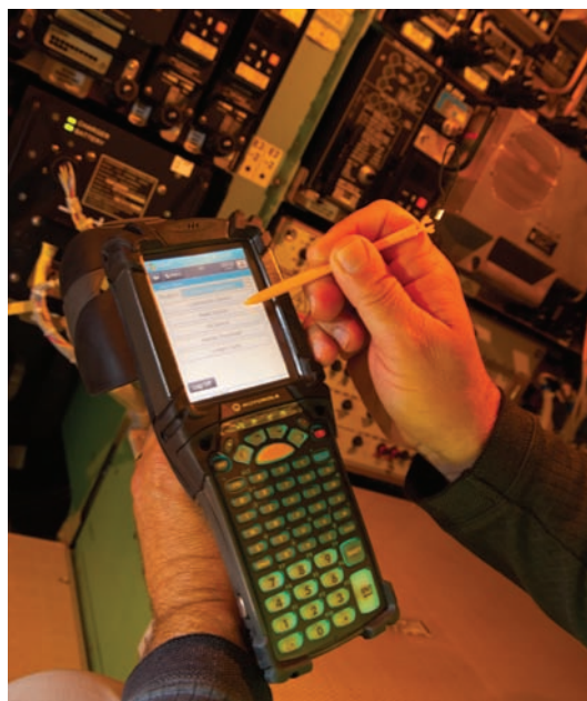
RFID tags emit a radio signal which is interrogated by a hand-held reader/writer device. Photo courtesy of The Boeing Company.
