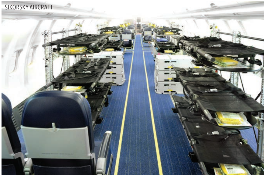
Fixed wing aircraft with stacking litter systems and stretcher interface module (SIM) units.
