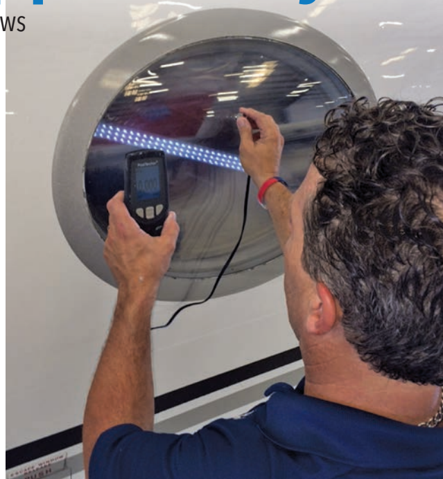
The aircraft windshield restoration process includes measuring each panel using ultrasound before and after to ensure it meets manufacturer's acceptable tolerances.
