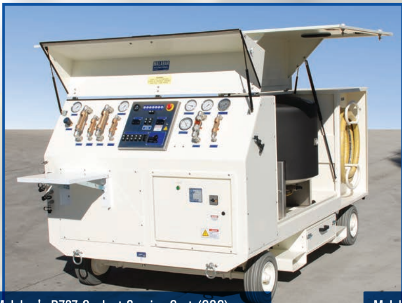
Malabar's B787 Coolant Service Cart (CSC) performs rapid aircraft coolant drain, fill, clean and de-aerate operations.
