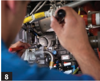
8 DALLAS AIRMOTIVE technician shown here inspecting a TFE731 engine. DALLAS AIRMOTIVE
