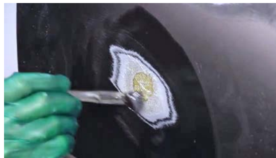
CARBON BLADE gouge repaired according to the manual. HARTZELL PROPELLER
