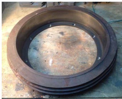
THE JUNKERS JU52 original brake drum (left), and the new one using reverse engineering (right).
