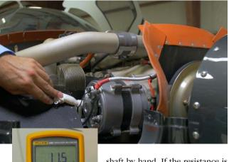
shaft by hand. If the resistance is high, not steady or infinite (using a calibrated VOM), you may have bad brushes, slip ring contamination, or an open rotor. If the resistance is "0": The field circuit is shorted, which makes the rotor suspect.
