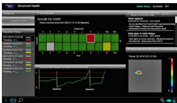
PULSE™ STRUCTURAL Health – Sample of cargo bay floor panel status. UTC AEROSPACE SYSTEMS
