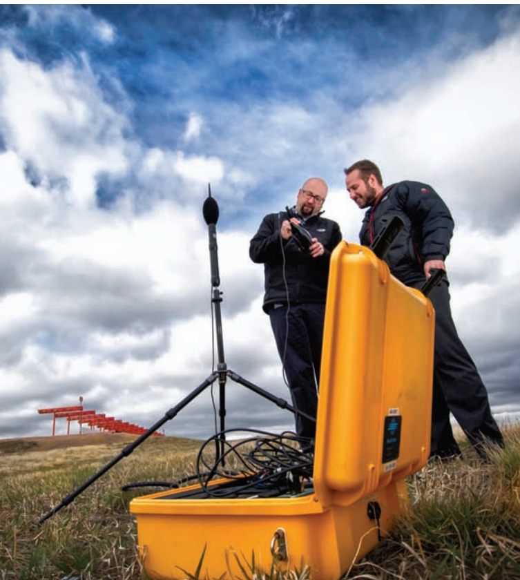
Portable noise monitoring systems, like this one used by Centennial Airport staff members Mike Fronapfel, left, and Aaron, right, help apply hard data to noise events to more accurately identify trends and anomalies.
