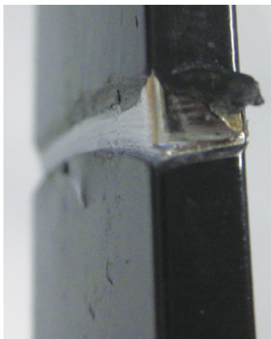
▲ Example of a shifter with a wear groove in the lever.
