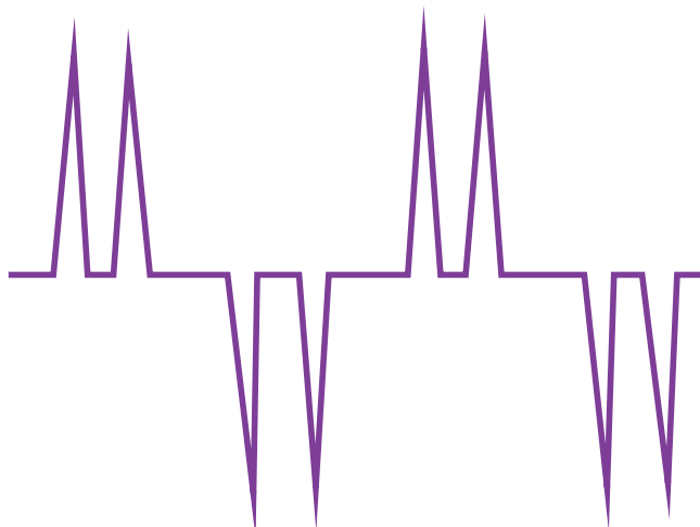
Figure 2 - Distorted waveform from 6-pulse VFD
