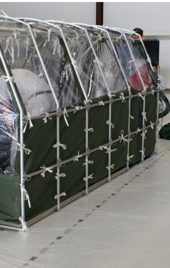
The Gulfstream III is modified from a 12-seat plane to a three-room chamber (antechamber, patient area, and small bathroom area).
