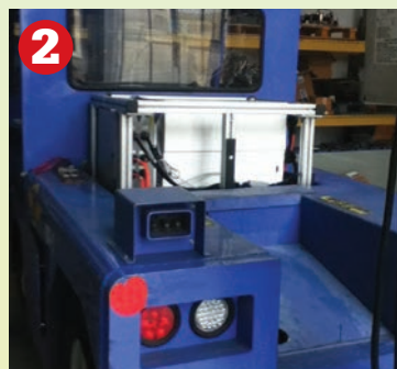
1. The Corvus lithium battery pack, with a specially designed container for the tractors. 2. A tractor integrated with the battery pack. 3. The Corvus battery integrated into a tractor with additional ballast weight for the six-month test.
