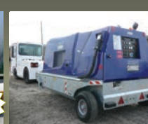
GUINAULT 90-180kVA GROUND POWER UNIT
