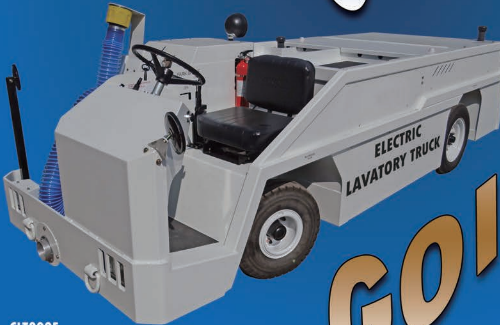
CLT200E 200 Gallon Capacity - Waste 100 Gallon Capacity - Water
