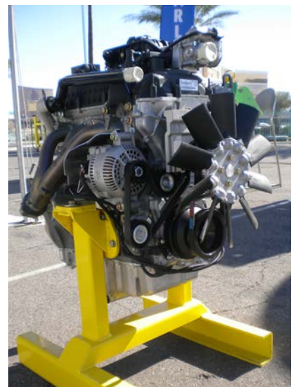
The CT5G can come with either this Ford four-cylinder, 2.5-liter engine or a four-cylinder, 2.8-liter engine from Zenith Power Products LLC.
