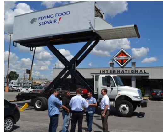
Global Ground Support supplied the rear body and scissor lift for the hybrid truck.
