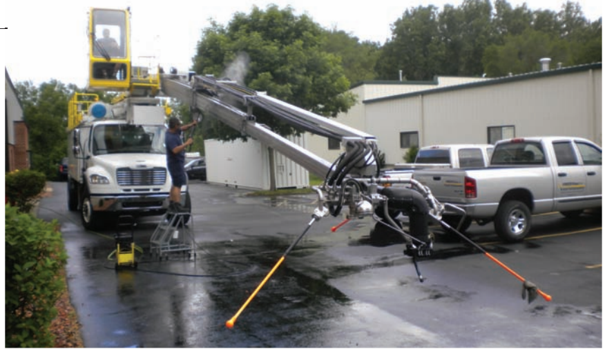
The key purpose of the telescopic boom is to bring the nozzle to a minimum distance from the aircraft for maximum deicing fluid efficiency, while keeping the deicer truck, its cabin and boom at a maximum distance from the aircraft for maximum safety.
