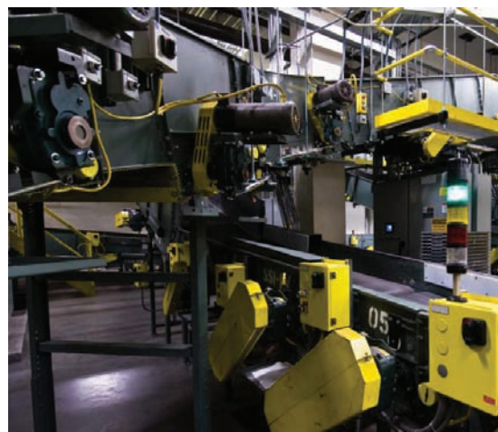
The baggage handling system at Fort Myers' Southwest Florida International Airport is certified to process 2,600 bags per hour through the L3 explosive detection systems (EDS) screening machines.
