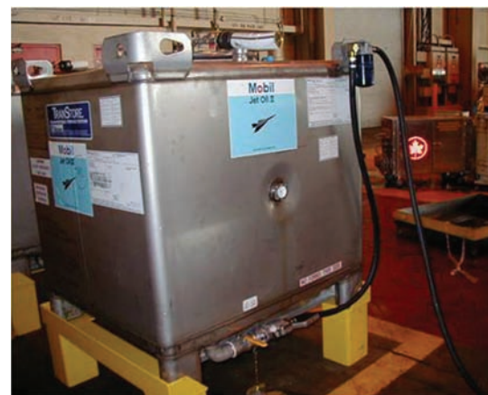
A compatible hose with a matching coupler is connected to the outflow port and compressed air or nitrogen power is used to transfer the oil from the tote to smaller containers.
