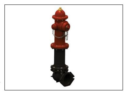
Finally, there are the drain holes. Drain holes are located in the foot-piece and open when the hydrant is shutdown allowing the water to escape from the barrel and prevent freezing during winter. On the other hand, these drain holes are sealed off when water is flowing, preventing erosion around the shoe.
