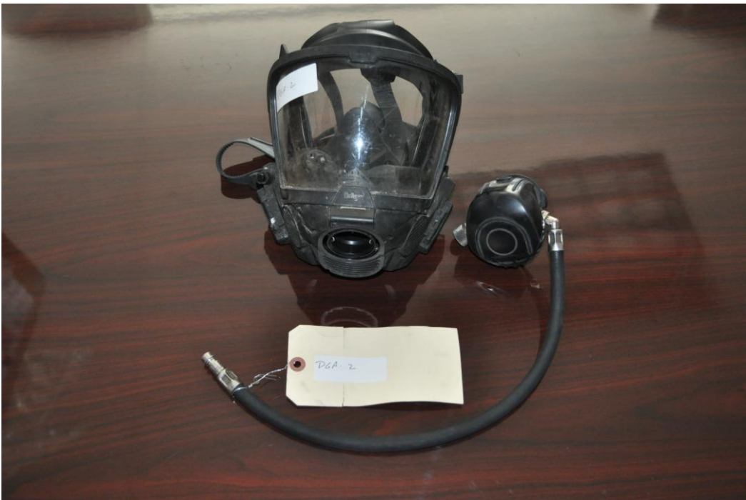
Figure 6 – DeKalb Unit #2 Facepiece and Second Stage Regulator
