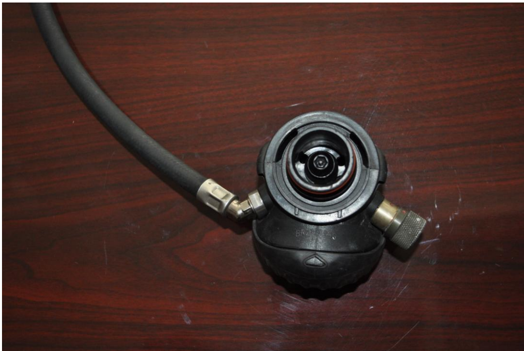
Figure 4 – DeKalb Unit #1 Second Stage Regulator Facepiece Interface Area
