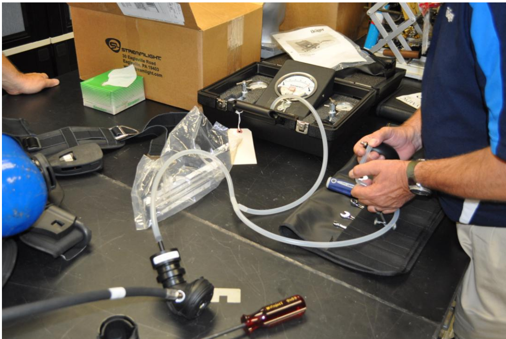
Figure 10 - Dräger Regulator Pressure Test Prior to NIOSH Testing
