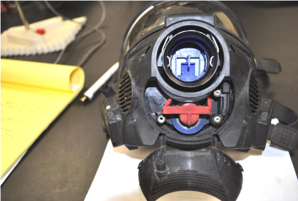
Figure 12 – DeKalb Unit #2 Facepiece Exhalation Valve Retainer and Spring
