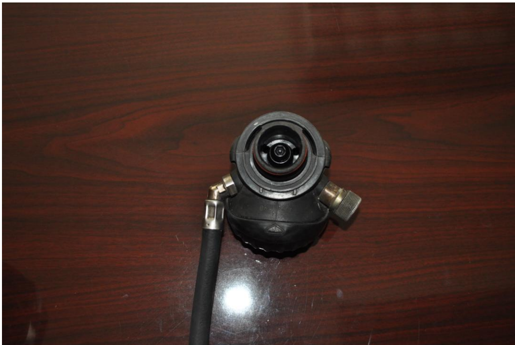
Figure 8 – DeKalb Unit #2 Second Stage Regulator Facepiece Interface Area
