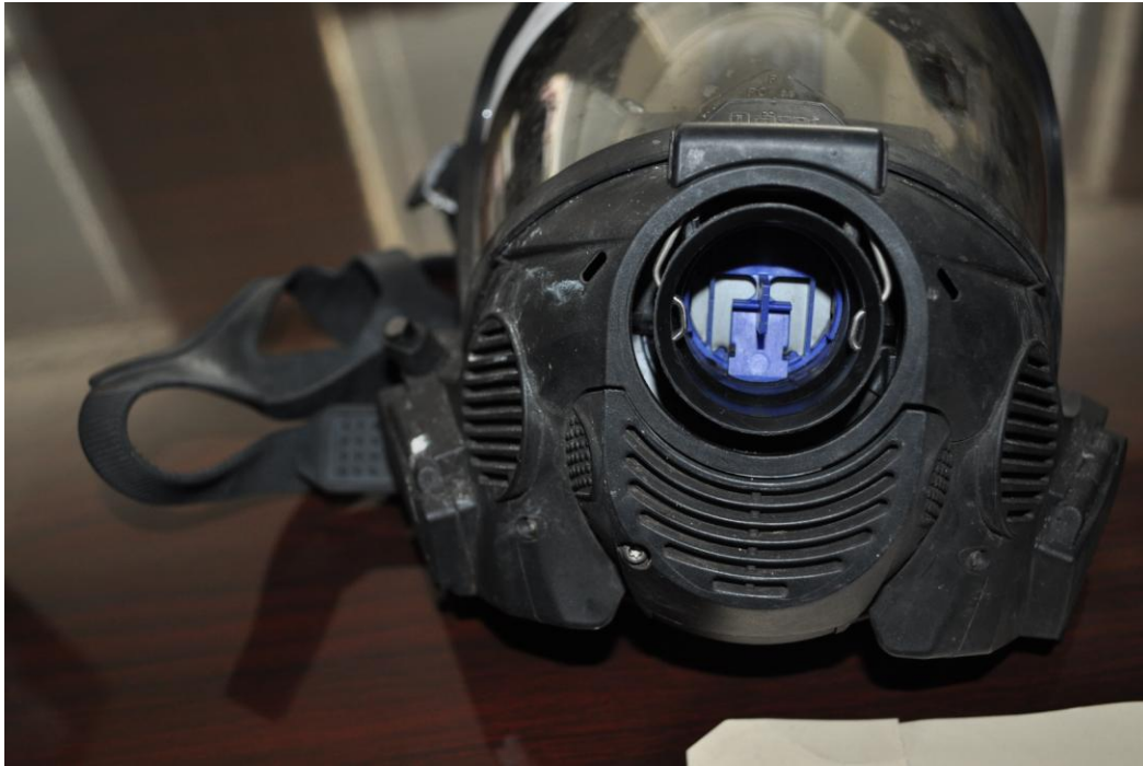
Figure 8 – DeKalb Unit #2 Second Stage Regulator Facepiece Interface Area
