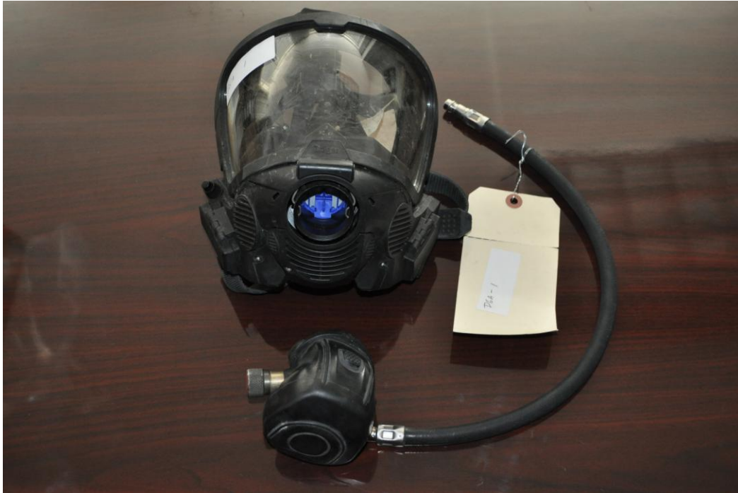
Figure 2: DeKalb Unit #1 Facepiece and Second Stage Regulator
