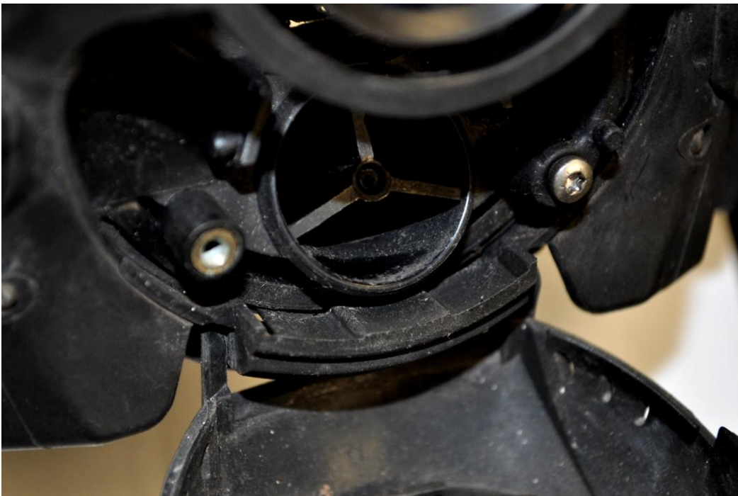
Figure 16 – DeKalb Unit #2 Facepiece Exhalation Valve Seat Area
