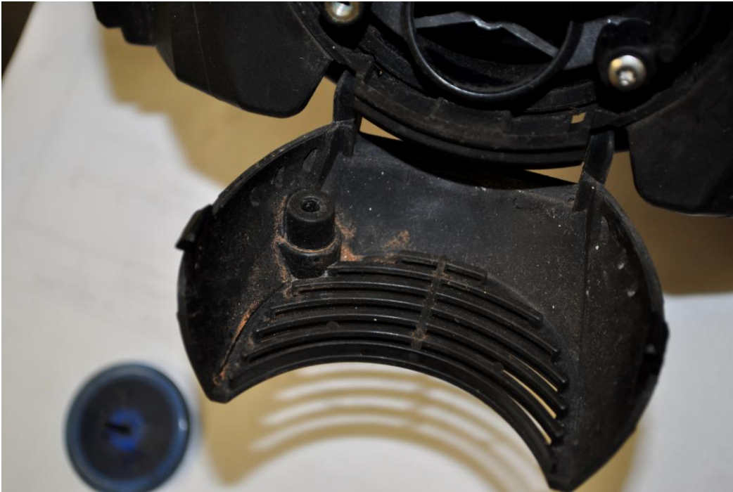
Figure 16 – DeKalb Unit #2 Facepiece Exhalation Valve Seat Area
