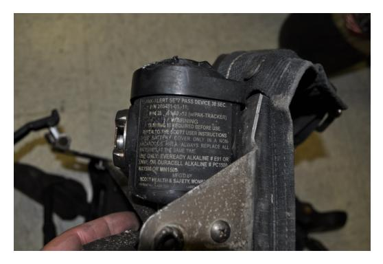
$Figure\ 26-Unit\ \#1\ Backframe\ with\ SEI/NFPA\ Labels,\ Straps\ and\ Additional\ Markings$
