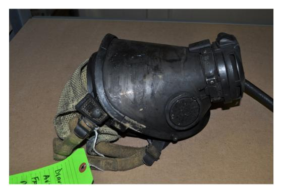
Figure 84 - Unit #3 Facepiece Regulator Interface Area
