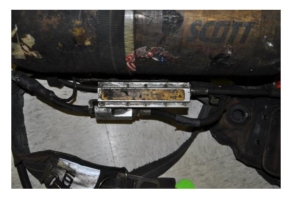
Figure 57 – Unit #2 High Pressure Hose and Cylinder Attachment with O-ring
