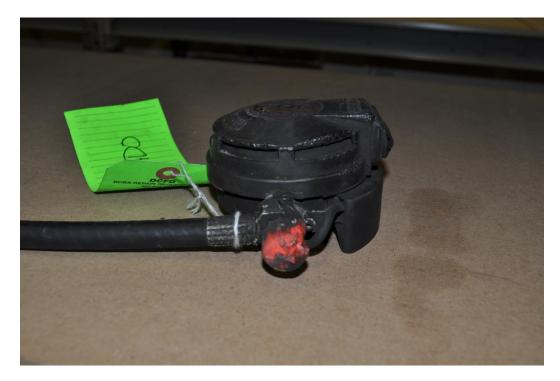
Figure 50 – Unit #2 Mask Mounted Regulator, Donning Switch
