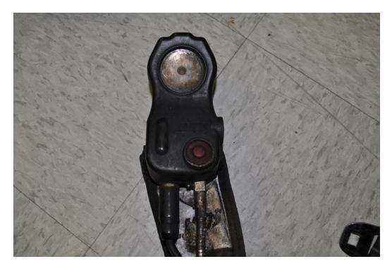
Figure 23 – Unit #1 Remote Gauge and PASS Console Back with SEI Label
