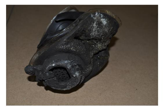
Figure 128 – Unit #4 Facepiece Inside View with Nose Cup
