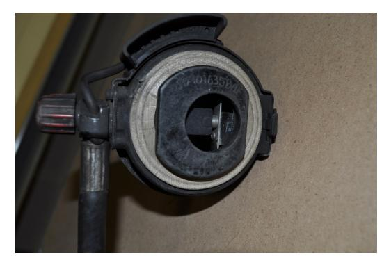
Figure 15 – Unit #1 Regulator and Low Pressure Hose with Quick Disconnect
