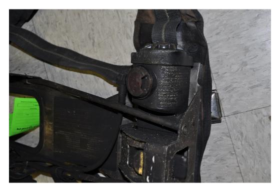
Figure 102 – Unit #3 Backframe Assembly without Cylinder
