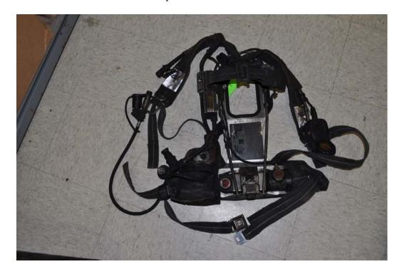
Figure 28 – Unit #1 Backframe with NIOSH Label
