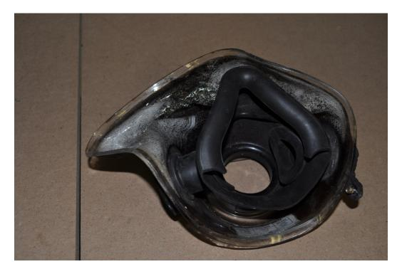
Figure 129 – Unit #4 Mask Mounted Regulator and By Pass Knob
