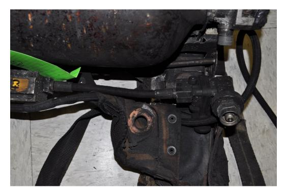
Figure 140 – Unit #4 Cylinder Connector with O-ring
