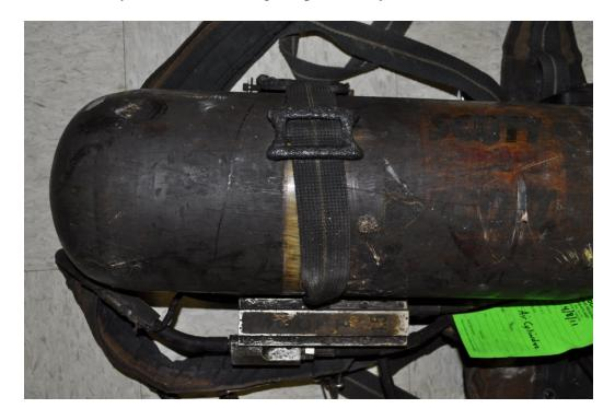
Figure 30 – Unit #1 Backframe with Cylinder Strap Assembly and Straps and Buckles
