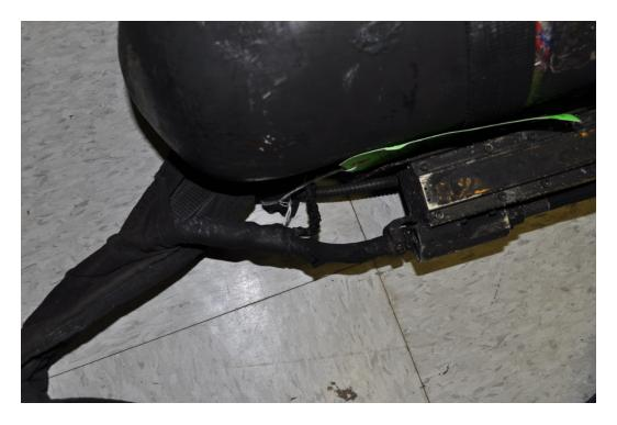
Figure 93 – Unit #3 Low Pressure Hose and HUD Wire
