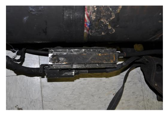
Figure 96 – Unit #3 High Pressure Hose and Cylinder Attachment Assembly
