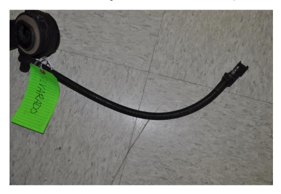
Figure 52 – Unit #2 Low Pressure Hose Quick Disconnect
