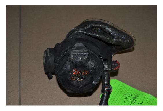
Figure 126 – Unit #4 Facepiece Regulator Interface Area
