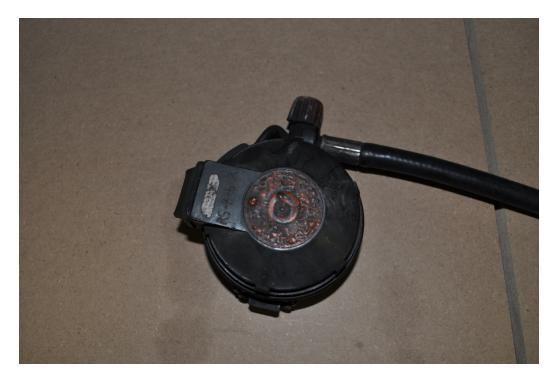
Figure 13 – Unit #1 Regulator, Donning Button, By-Pass and HUD Assembly
