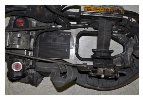
Figure 63 – Unit #2 Backframe and Cylinder Strap Assembly
