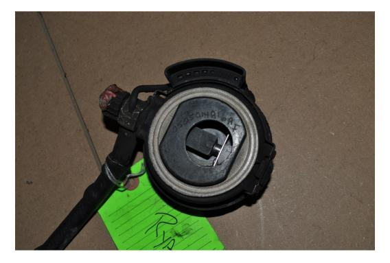
Figure 132 – Unit #4 Low Pressure Hose Attachment to Regulator
