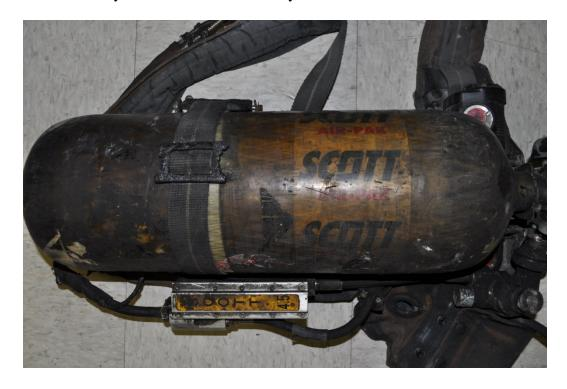
Figure 71 – Unit #2 Cylinder Assembly with Labels
