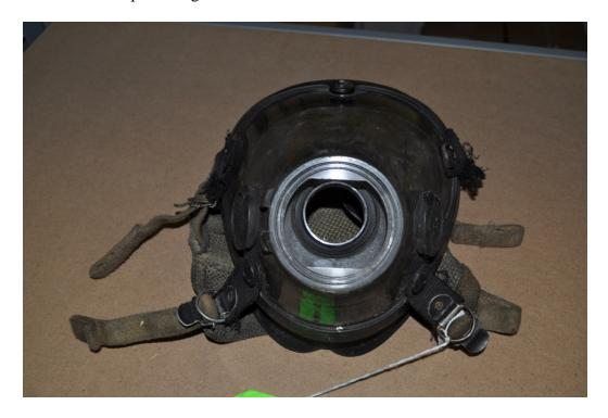
Figure 8 – Unit #1 Facepiece Right Side with Torn Strap Attachment
