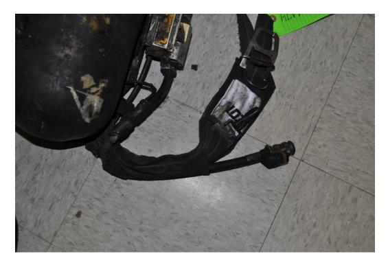
Figure 54 – Unit #2 Hose Connections to Pressure Reducer
