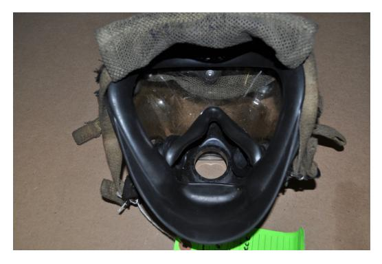
Figure 11 – Unit #1 Facepiece View Through Lens
