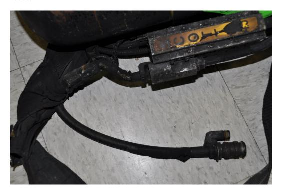
Figure 137 – Unit #4 High Pressure Reducer and Hose Connections
