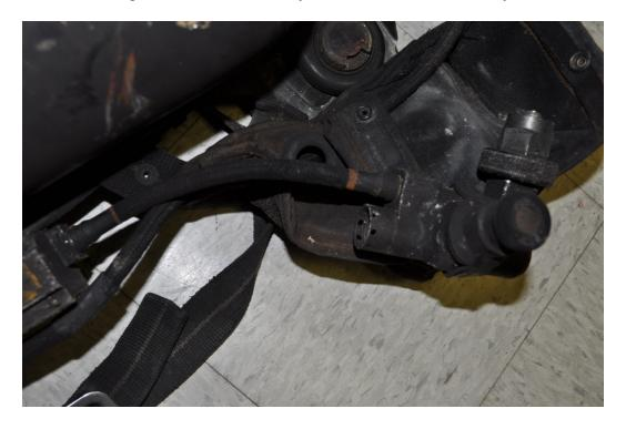
Figure 97 – Unit #3 Cylinder Connection with Relief Valve Top Missing
