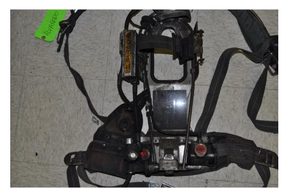
Figure 68 – Unit #2 Left Shoulder Adjustment Strap Wear
