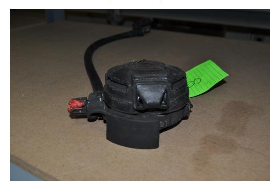
$Figure\ 51-Unit\ \#2\ Mask\ Mounted\ Regulator\ with\ Low\ Pressure\ Hose\ and\ Quick\ Disconnect$
