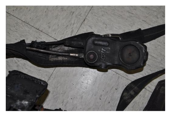
Figure 142 - Unit # 4 Remote Gauge and PASS with Damaged SEI Label
