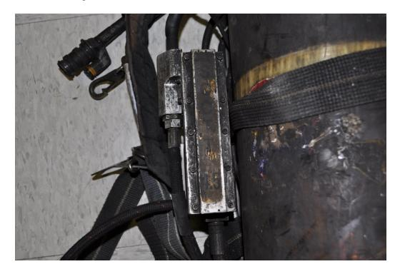
Figure 20 – Unit #1 High Pressure Reducer Side with Hose Attachments
