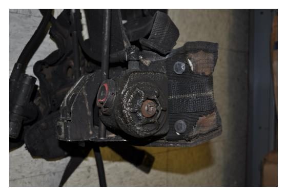
Figure 145 – Unit #4 HUD Wire and Low Pressure Hose Assembly
