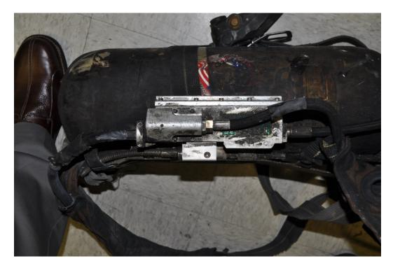
Figure 56 - Unit #2 Pressure Reducer with Hose Connections
