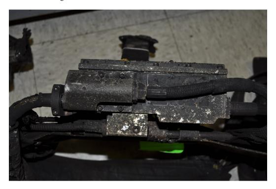
Figure 139 – Unit #4 High Pressure Hose and Cylinder Connection
