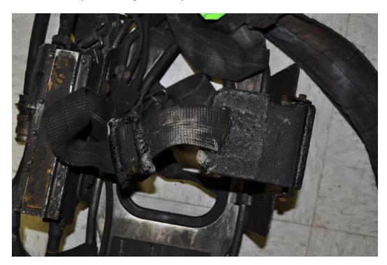
Figure 105 – Unit #3 Backframe Assembly with NIOSH Label After Cleaning
