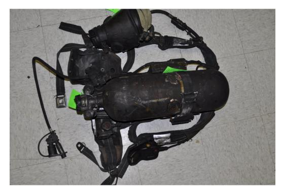
Figure 82 – Unit #3 Facepiece and Mask Mounted Regulator Assembly
