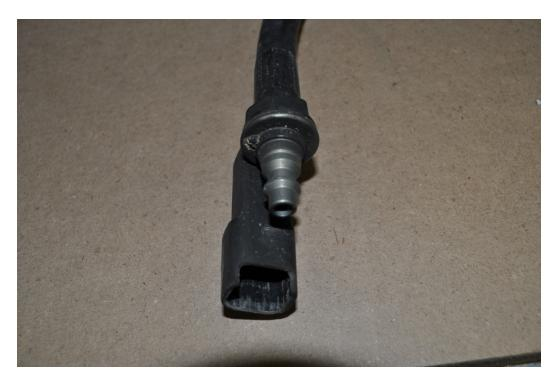
Figure 53 – Unit #2 Low Pressure Hose with Quick Disconnect and Connection to Pressure Reducer
