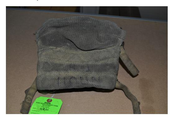
Figure 10 – Unit #1 Facepiece Nosecup and Inside View
