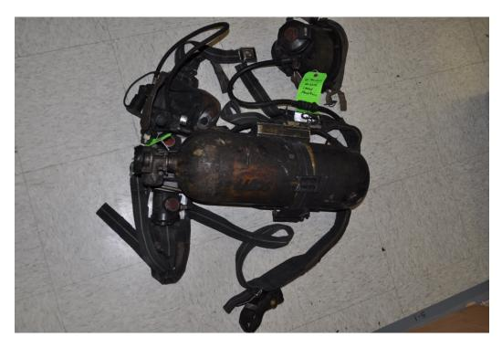
Figure 5 – Unit #1 Facepiece with Mask Mounted Regulator Attached
