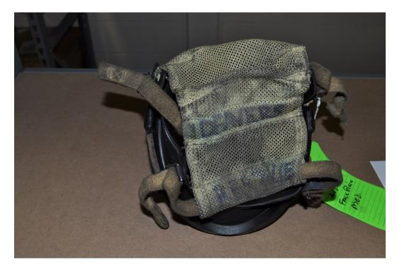
Figure 86 – Unit #3 Facepiece Inside View and Nose Cup
