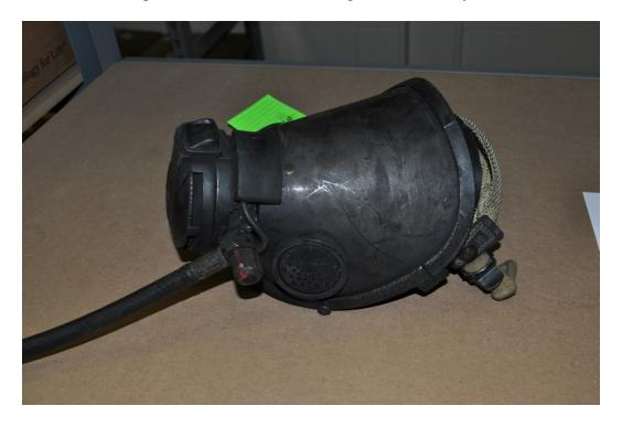
Figure 83 – Unit #3 Facepiece and Regulator Assembly, Facepiece Damage
