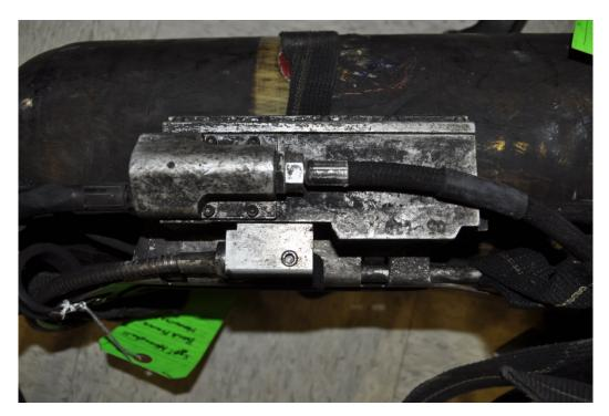
Figure 21 – Unit #1 Cylinder with Cylinder Attachment, O-ring and High Pressure Hose
