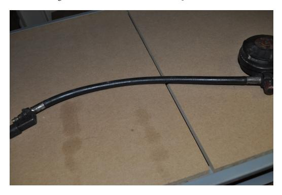
Figure 16 – Unit #1 Low Pressure Hose Quick Disconnect
