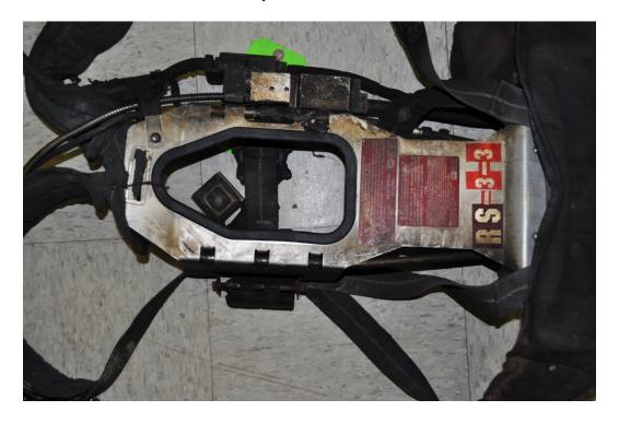
Figure 147 – Unit #4 Cylinder Strap Assembly
