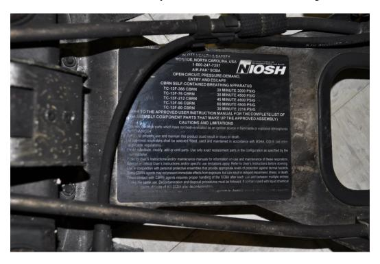
Figure 106 – Unit #3 Backframe Assembly with SEI/NFPA Labels
