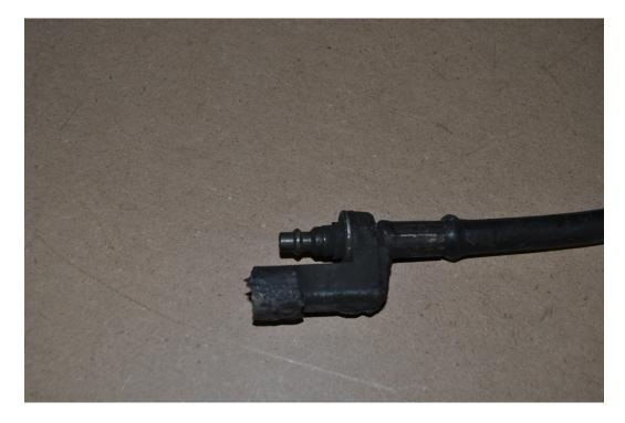
Figure 136 – Unit #4 Low Pressure Hose and Quick Disconnect, Attached to High Pressure Reducer
