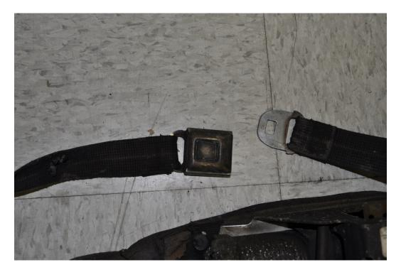
Figure 152 – Unit #4 Left Shoulder Adjustable Strap with Damage
