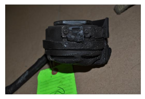
Figure 131 – Unit #4 Regulator Inside View
