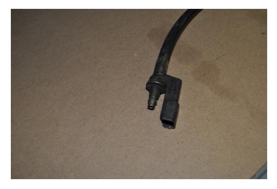
Figure 17 – Unit #1 Low Pressure Hose with Quick Disconnect
