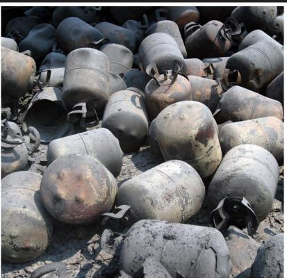
plug remain intact after exposure to fire, do not attempt to move the cylinder until it has been allowed to reach ambient temperatures, as the acetylene may be decomposing internally and the cylinder is still subject to a violent failure!
