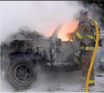
The fuel tanks being used today are plastic, and can quickly melt should the fire extend under the chassis. When this occurs, fire can spread rapidly engulfing the vehicle and in some cases igniting exposures. Keep in mind that the fuel tank is located just under the trunk on many vehicles.
