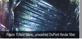
A closer look at an outer shell under a microscope shows non-fibrillated DuPont Kevlar fiber (Figure 1) and fibrillated DuPont Kevlar fiber (Figure 2). After fibrillation the fiber reflects light in a different cast. Darker fabrics like black shift from a rich dark color to charcoal; lighter fabrics such as gold may develop a hairy appearance.
