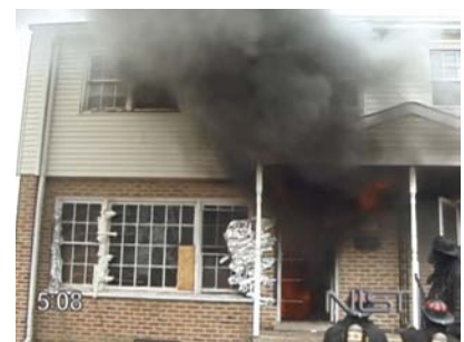
5:08: The fire department forces the front door and prepares to make entry. Fire receives a rush of fresh air through the open front door (flow path) and rapidly returns to the free burning state eventually reaching flashover conditions.
