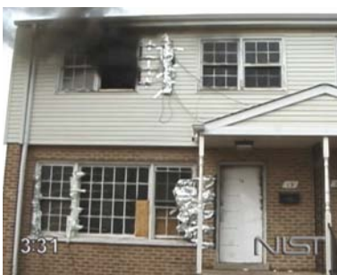
NIST research captured fire development in a burn building. 3:31: Fire is free-burning prior to the fire department's arrival. Notice outward signs of smoke indicating a free-burning fire with plenty of oxygen.
