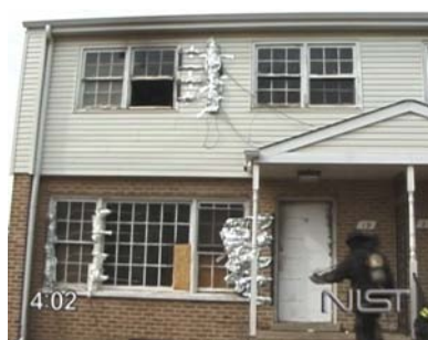
4:02: The fire department arrives on scene. Fire has become ventilation-limited, causing a reduction of pressure inside the building and little to no outward signs of smoke are visible. Images Courtesy NIST
