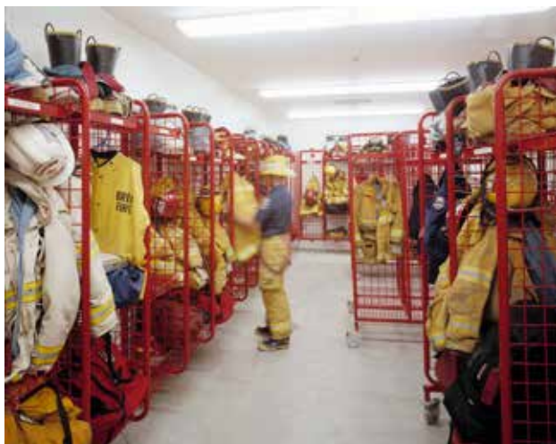
Turnouts should be stored as far from the living quarters as possible to protect firefighters from off-gassing of harmful contaminants.
