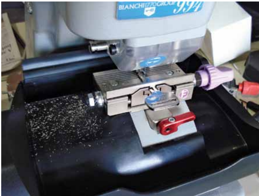
Key inserted into the 'F' jaw
