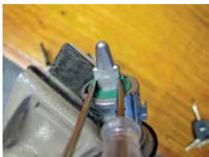
Photo 28. Use 2 small screwdrivers to gently lift tabs on plastic clip & slide clip off.
