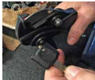
Key Head Cut Down To a Manageable Size
