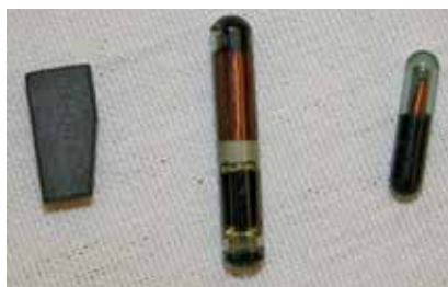
Transponder Chip, Large Ampoule and Smaller Ampoule
