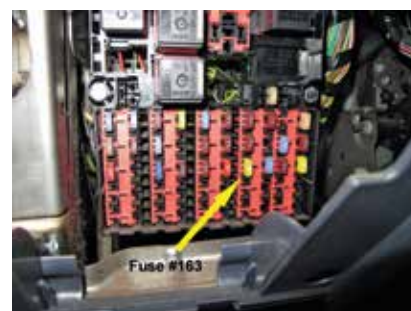
Photo 24. Power door lock fuse is #163.
