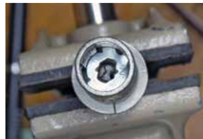
Photo 36. Lug on inside of chamber must fit between the two stops on the disc.
