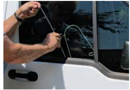
Photo 7. Remove wedges before pulling tool up inside the vehicle
