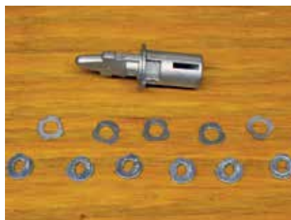
Photo 12. Full set of discs & spacers from 6-disc Tibbe lock.
