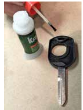
Place Glue Around Outer Lip of Interior Housing
