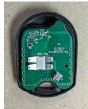
Circuit Board Placed over Rubber Pushbutton Pad in Front Cover
