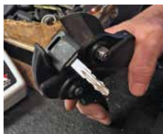
Cutting Off Head portion Above Key Ring Opening
