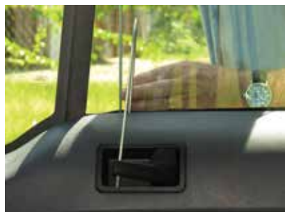
Photo 9. Pushing shaft of tool forward will push handle out & unlock door.
