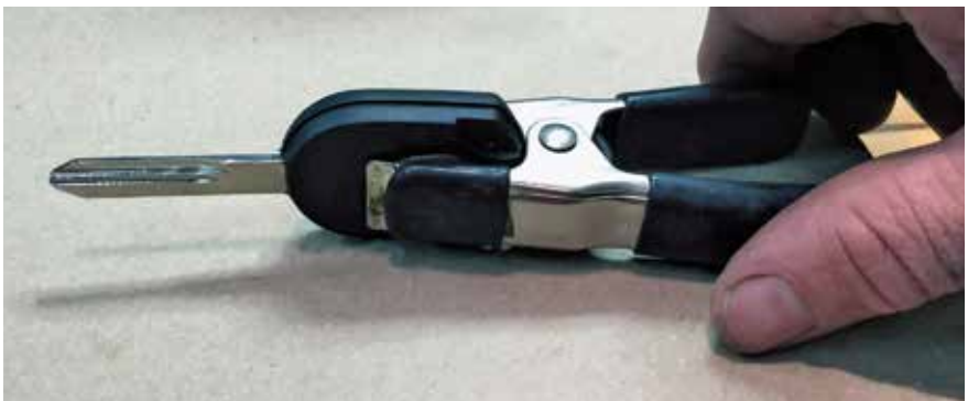
Use Two One-Inch Clamps to Secure Shell for Drying
