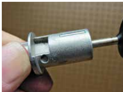
Photo 17. Lock with correct key inserted & turned, allowing sidebar to drop into unlocked position.
