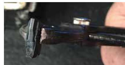
Breaking open Encapsulation to Expose Transponder Chip
