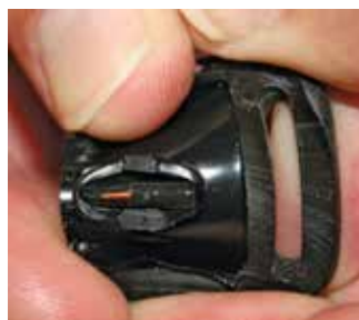
Removing transponder ampoule, closeup view
