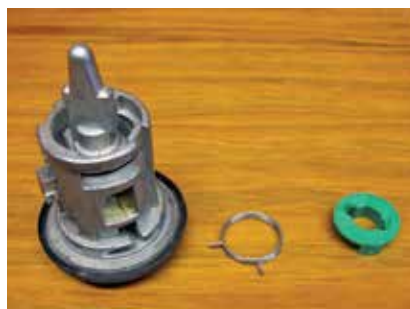
Photo 29. Return spring wound around plastic clip will come free of lock.
