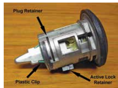
Photo 27. Lock removed, showing one of the slots that engage with lugs as well as part of plug retainer and plastic anti-rattle clip.
