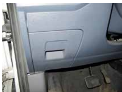
Photo 23. If equipped with power door lock, fuse is behind panel on left side of dash.
