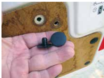
Photo 19. Fiberboard trim panel secured with 11 upholstery clips.
