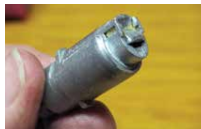
Photo 43. Shutter assembly is permanently attached to lock chamber, which prohibits further disassembly.
