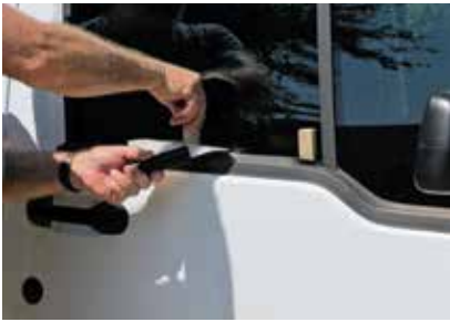
Photo 4. Plastic shim protects weatherstripping as wedges are inserted
