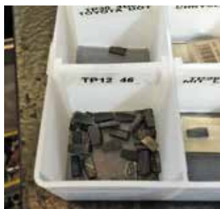
Harvested Transponder Chips
