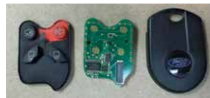
Original Rubber Pushbutton Pad, Circuit Board and Logo Rear Cover
