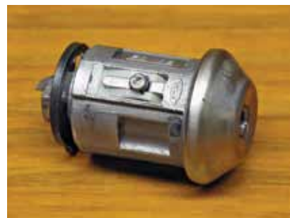
Photo 39. Lock cylinder removed from column.
