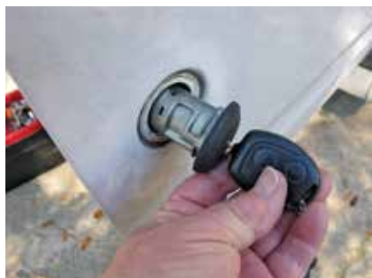
Photo 25. Once the active retainer has been depressed, rotate lock counter-clockwise & pull free of door.
