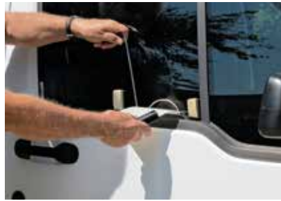
Photo 6. Shim used again to protect weatherstripping as tool is inserted.
