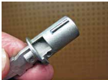
Photo 16. Lock with incorrect key inserted & sidebar in raised position
