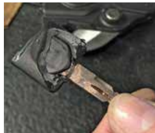
Transponder Covering Exposed
