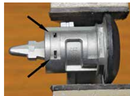
Photo 30. 2 ends of horseshoe plug retainer.
