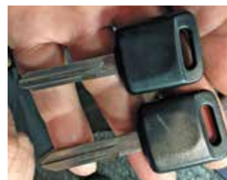
Two Nissan Transponder-Equipped Key Blanks. NA is stamped onto blade on obverse side only
