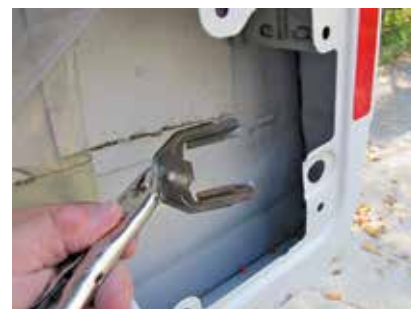
Photo 21. Anti-rattle clip removed with pliers.
