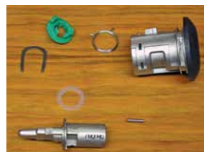
Photo 33. Lock cylinder components.
