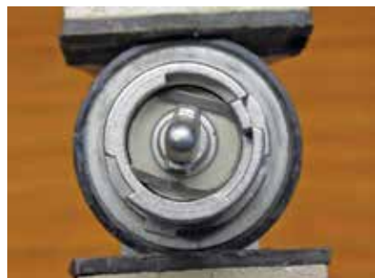
Photo 31. Horseshoe retainer as seen from rear of lock.
