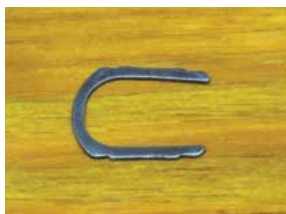
Photo 32. Horseshoe retainer removed from the lock.
