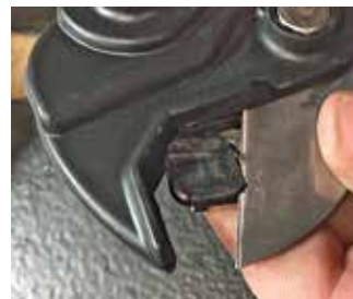
Removing Encapsulated Transponder from Blade
