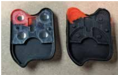
Customer's Rubber Pushbutton Pad with Contact in place and Replacement Rubber Pushbutton Pad
