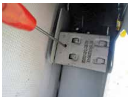
Photo 22. Use an ice pick or similar tool to access the active retainer through the poke-hole
