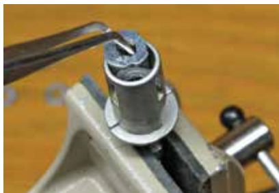
Photo 35. Discs placed in chamber with numbered sides up & a spacer between each disc.
