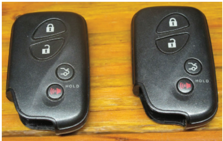
Photo 2. Two apparently identical prox fobs for a 2012 Lexus IS-250. One has the older circuit boards and the other has the newer replacement circuit board. The information stamped on the outside of the case may not be correct and should be ignored.
