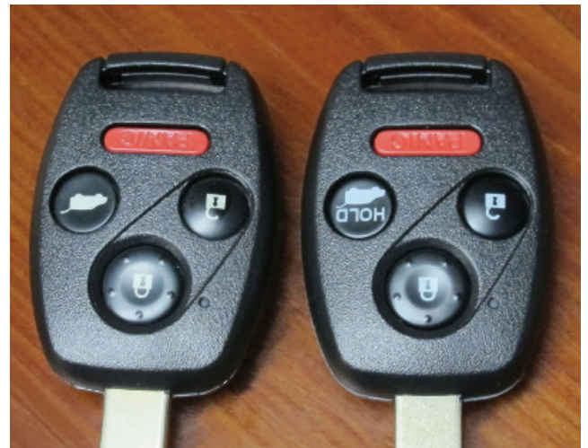
Photo 1. Two nearly identical Honda Pilot IRKs. The key on the left releases the rear glass in the hatch, while the key on the right operates the power opening and closing of the entire hatch.
