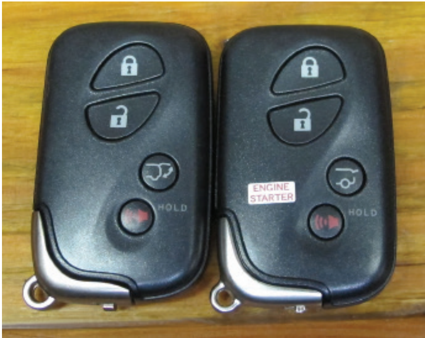
Photo 5. Another set of nearly identical, but not interchangeable Lexus prox fobs. The fob on the left is intended for SUVs that have a powered rear hatch. The fob on the right is intended for vehicles without a powered rear hatch, and releases the glass portion of the rear hatch.
