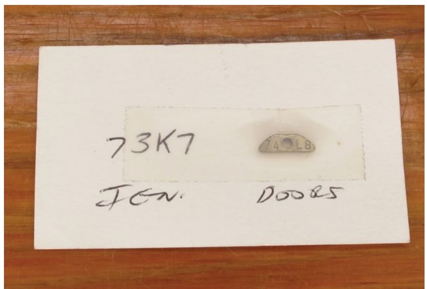
Image 4: I found this card in the glove box of an old Buick that was equipped with VATS. I replaced it with my business card and included the VATS resistor value for the car.
