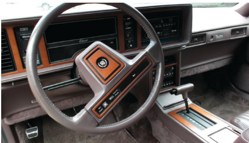
Image 2: A Canadian-made steering column was on certain Buick and Cadillac models. Notice that the cruise control is on the horn pad rather than the turn signal stalk.
