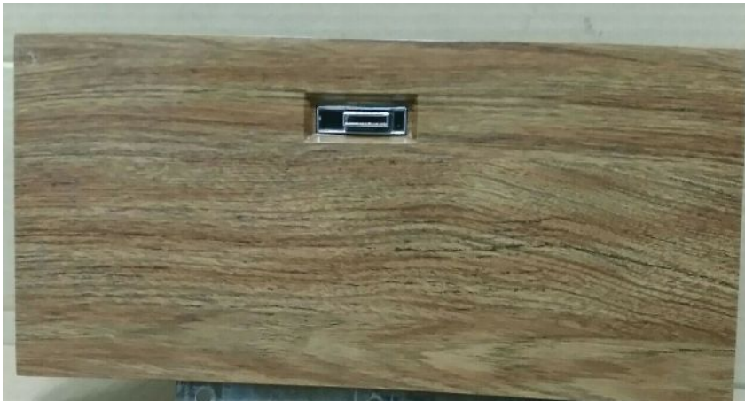
Image 3: This unusual glove box lock slides from right to left and was used on only a few high-end vehicles, such as the Cadillac Seville and Eldorado. It's a full six-cut lock, so a complete door key can be made from it. But if it's locked, it's a real pain to access.
