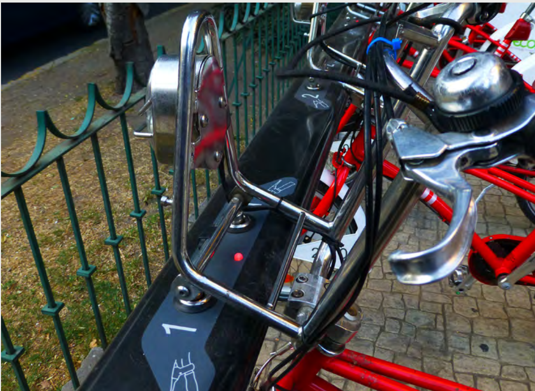
TOP In Rio de Janeiro's system, bikes lock into the side of the docking bar, rather than the top.
