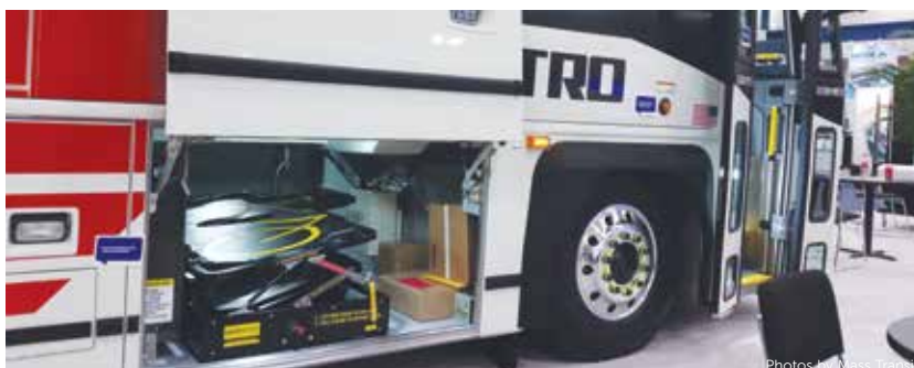
THE MCI buses for Metro include a Sportswork bike rack where the luggage compartment is on a coach, protecting the bikes on highway driving.
