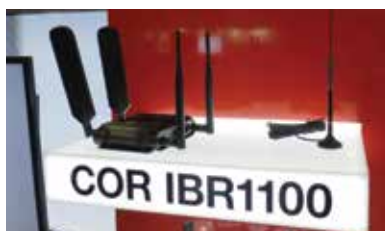
THE CRADLEPOINT COR IBR1100 is fully ruggedized to military specs and features 4G LTE capabilities.
