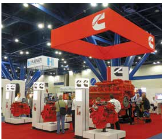
THE QSK95 16-cylinder 95L engine provides up to 4,440 HP.
