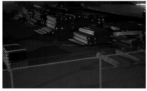
As the light level decreases, Avigilon cameras with Day/Night technology remove the infrared (IR) cut filter in order to use all sources of ambient light to capture as much detail as possible in monochrome (black and white).
