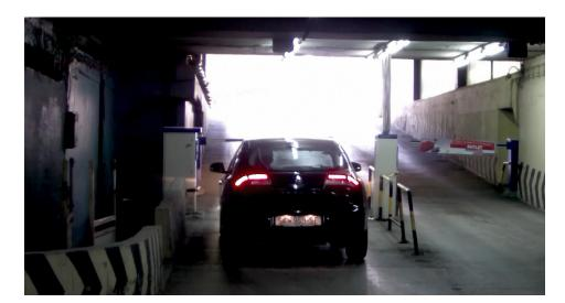
In environments experiencing a high range of illumination, cameras without WDR technology will not be able to detect details in portions of the image, as bright parts will be oversaturated, and dark parts will be too dark (left corner).
