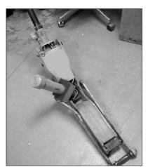
When the pressure of the load was placed on the jack, the bolt "blew out" and the load collapsed. Luckily no one was hurt and the forklift was not damaged. But the costs could have been greater. Had someone routinely given the jack a "look over" he may have noted the bolt not completely seated and prevented the accident.
