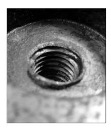
Momentarily after lifting a very large forklift, there was a loud bang and the load dropped. Upon further investigation, it was determined that a bolt had backed out of the threads and when the lifting began, the bolt was only being held by a thread or two.
