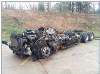
A burnt truck from a poor inverter installation.
