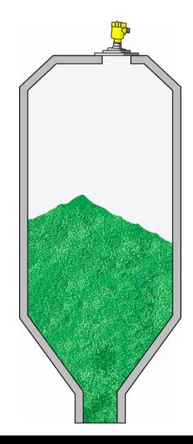
**80-GHZ RADAR** Figure 1. An 80-GHz radar can more accurately detect and measure polyethylene flakes in silos or storage bins.
