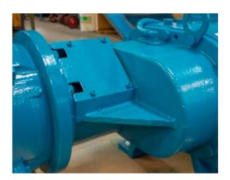
C-FLANGE SETUP Figure 2. A C-flange setup allows for a direct-drive motor to be connected, and saves space while eliminating belt and sheave issues.
