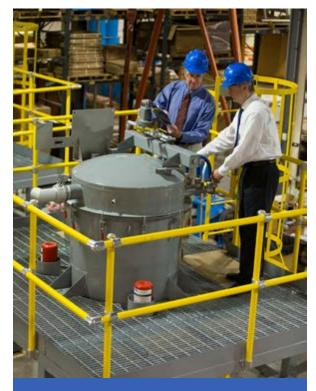
CENTRAL VACUUM CLEANING Figure 2. System for continuous dust control helps reduce the possibility of dust explosions as well as respiratory, slip and ergonomic hazards.
