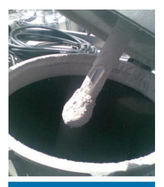
**DROP ANTENNA** Figure 3. The drop antenna shape is unaffected by powder buildup, resulting in reliable signal strength.
