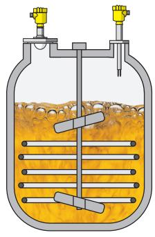
Rotating agitator blades take up a lot of real estate and do not leave much room for a microwave beam to emit from a radar antenna, hit the product surface, and reflect back to the antenna without interference. The beam angle was just too wide. That is, until 80 GHz radar sensors hit the scene. These higher frequency devices produce a beam angle as narrow as 3°. This unrivaled focus makes it possible to use a through-air radar level sensor on a reactor, even as the agitator spins.
