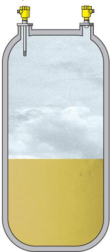
Chlorine measurement gives us the opportunity to discuss another way through-air radar sensors are rising to the challenges of modern chemical production. Chlorine is one of many liquids that is chemically difficult to measure, often due to a low dielectric constant. Liquids with a low dielectric constant—chlorine's dielectric value is 2—do not reflect radar signals well, making them resistant to radar technology. This resistance, however, can be overcome with large dynamic range.
