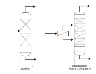
MEMBRANE/DISTILLATION HYBRID Figure 3. Using a membrane as a prefractionator frequently can provide substantial energy savings.
