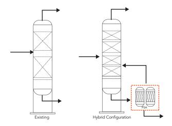
DISTILLATION/ADSORPTION HYBRID Figure 4. An adsorber can enable reintroducing a light component at an optimum location in a column, lowering energy consumption.
