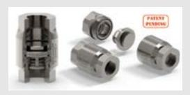
contoured surfaces with a minimum change in direction. The check valve also achieves a high flow capacity and reduced pressure loss compared to other poppet style check valves of similar sized connections. These features minimize the pressure drop across the valve. The valve closes quickly and smoothly for silent operation and eliminates water hammer.
