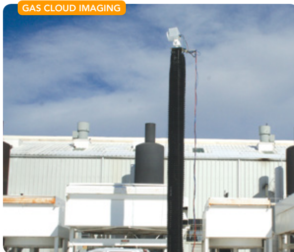
Figure 4. Camera can identify specific hydrocarbons and also generate a leak rate. Source: Rebellion Photonics.
