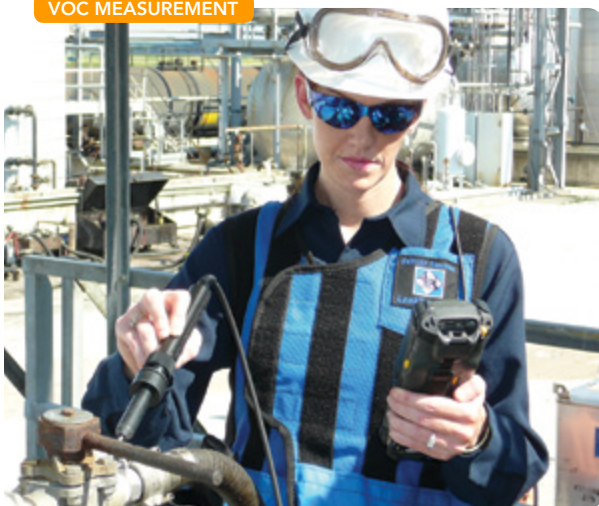
Figure 3. Current sniffing technologies for monitoring volatile organic compounds rely on a probe with a small diameter. Source: Team Industrial Services.
