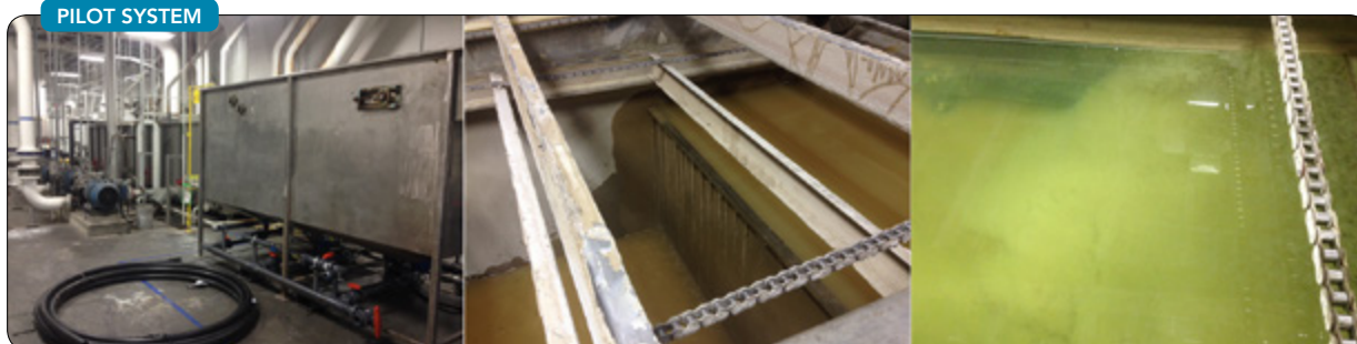
Figure 2. Once the customized pilot system was set up, the operator filled the tank with process water and began treatment using the chemical formula determined in stage 1.
