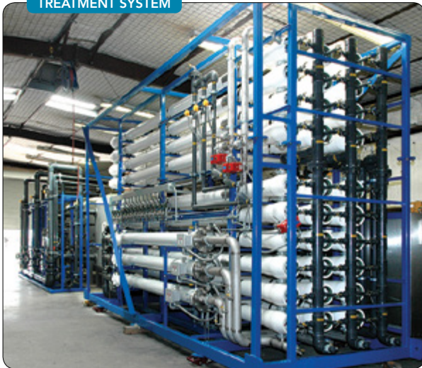
Figure 1: A large, compact skid with reverse osmosis (RO) technology meets regulations, reduces chemical costs and requires less overall maintenance.
