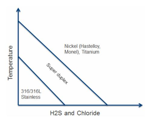
NACE specifications are detailed and can be complex when addressing combinations of variables. Regardless, they are important and necessary requirements for the safe measurement and control of raw, corrosive gas and oil that have been extracted from the ground or seabed.
