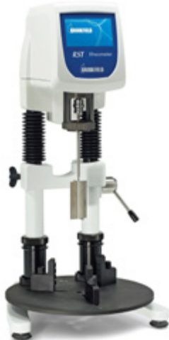
Figure 4: This rheometer has a much broader torque range capability compared to a viscometer.
