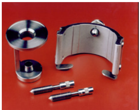
Figure 3. This vane spindle simulates augur mixing and measures viscosity at different rotational speeds, providing data similar to the graph shown in Figure 2.
